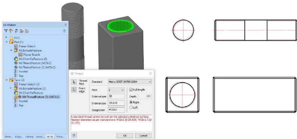
In projection views of 3D models with a thread, obtained by projection onto a plane parallel to the axis of the thread, the thread is indicated by thin lines. In projection views of 3D models with a thread, obtained by projection onto a plane perpendicular to the axis of the thread, the thread is indicated by an arc  $\frac{3}{4}$  of a circle.
